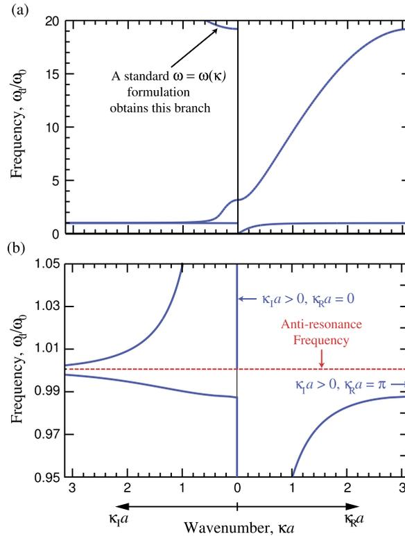
**Fig. 2.** Undamped band structure of the locally resonant metamaterial of Fig. 1a. (a) Uppermost branch is obtained by a standard  $\omega = \omega(\kappa)$  formulation as well as by the proposed algorithm, thus providing a verification on the accuracy of the algorithm. (b) Illustration of wavenumber subsegments inside the band gap. Separated by an anti-resonance frequency, the lower subsegment has  $\kappa_R = \pi/a$  and the upper subsegment has  $\kappa_R = 0$ .
