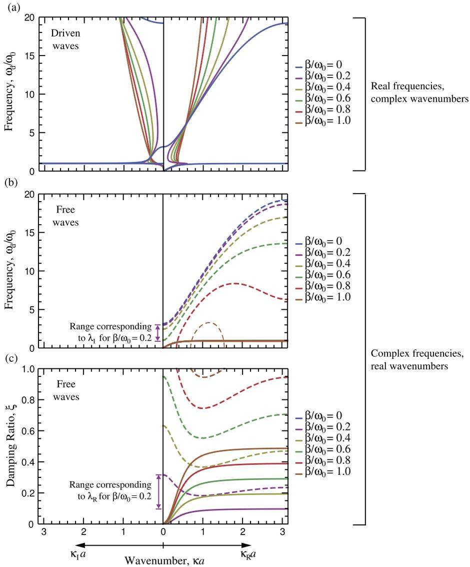
**Fig. 4.** Dispersion curves. (a) The frequency band diagram for driven waves generated by direct solving of  $\kappa = \kappa(\lambda)$  where, for  $\beta/\omega_0 > 0$ ,  $\kappa$  is complex for all prescribed  $\lambda = i\omega$ . The incomplete frequency (b) and damping ratio (c) band diagrams for free waves generated by direct solving of  $\lambda = \lambda(\kappa)$  for all prescribed  $\kappa = \kappa_R$  where  $\kappa_R \in [0, \pi/a]$ .
